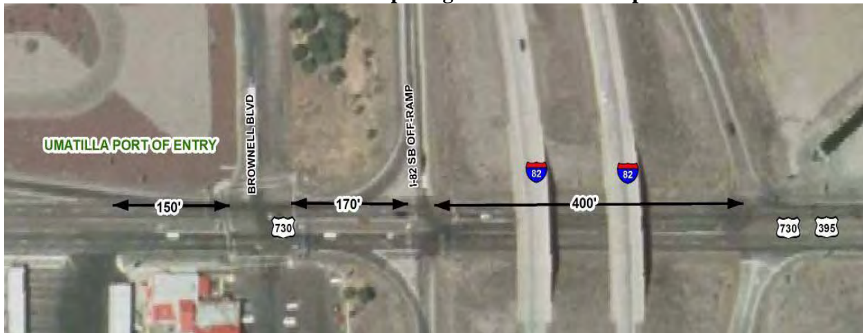
Exhibit 12.3-1 Intersection Spacing Near I-82 SB Ramp Terminals
